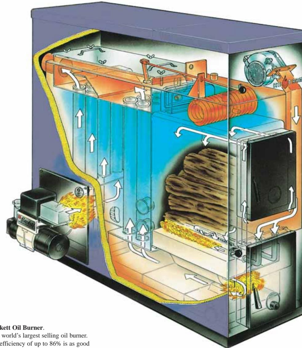
▼ **Beckett Oil Burner.** The world's largest selling oil burner. Oil efficiency of up to 86% is as good or better than most single fuel boilers.
