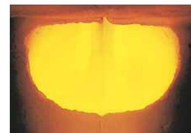
▼ **Combustion Tunnel.** This is where the magic of "wood gasification" occurs. This is the view you will get when you look into the observation port on the lower door. Temperatures of over 2000 degrees are achieved, therefore utilizing all available energy in the wood.
