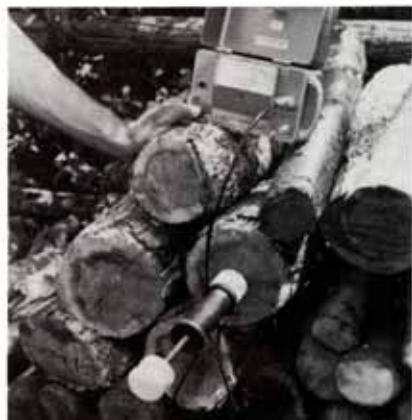
Meter reads 23-percent moisture content in logs seasoned for 10 months—slightly high for clean burning.
