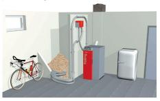
**Universal Suction**—one or three suction probes uniformly provides complete emptying of the pellet store room.
