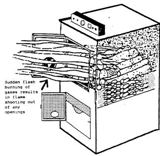
Following the recommendations in this manual will minimize the possibility of overheating, but even the most experienced person will occasionally overheat his boiler. To cope with this problem, the boiler is equipped with two safety devices-the Overheat Control and the Pressure Relief Valve.
