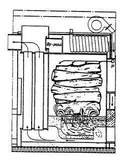
Correct amount of secondary air the flame is adaquate and does not smoke.
