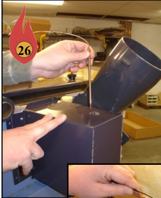
Install Lo-Limit Probe Use Right Wire Channel to Hide Tubing
