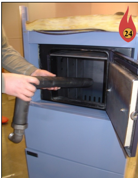
Remove Supply Pipe Assembly from Boiler
