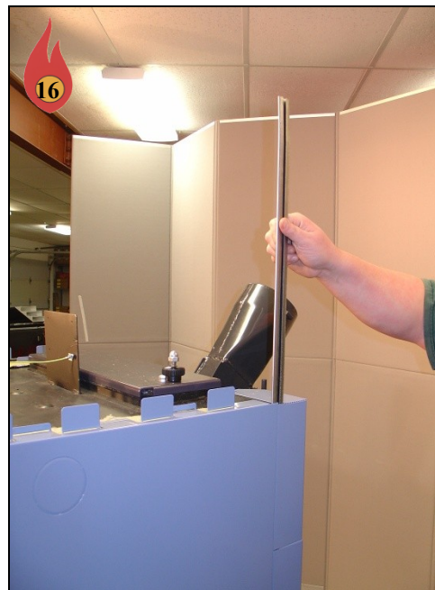
Install Right Rear Corner Zip Strip
