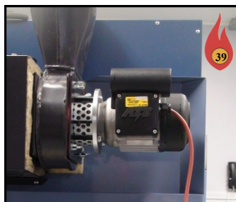
Mount Fan on Housing
