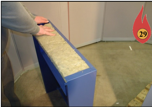
Install Insulation on back of top panel.
