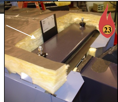
Install Insulation Blanket
