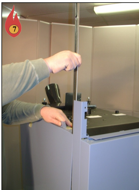
Install Left Front Corner Zip Strip
